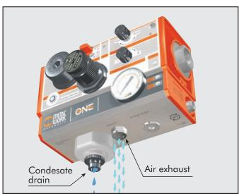
The air in the circuit is relieved via one outlet situated below the unit and fitted with silencer. If you want to convey air relief to prevent the emission of polluted air into the atmosphere, you can replace the silencer and install a fitting. (a pipe with a diameter of at least 6 mm is recommended)
